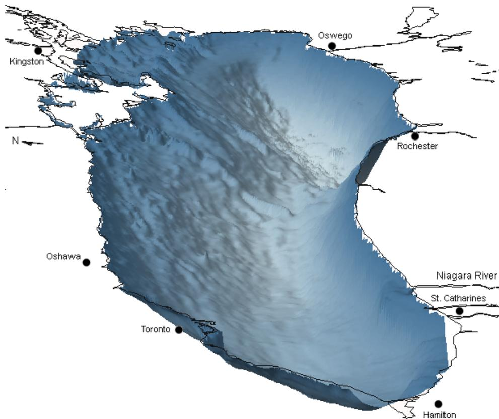
**Fig. 8:** Bathymetry Data Model for Lake Ontario (west perspective)
