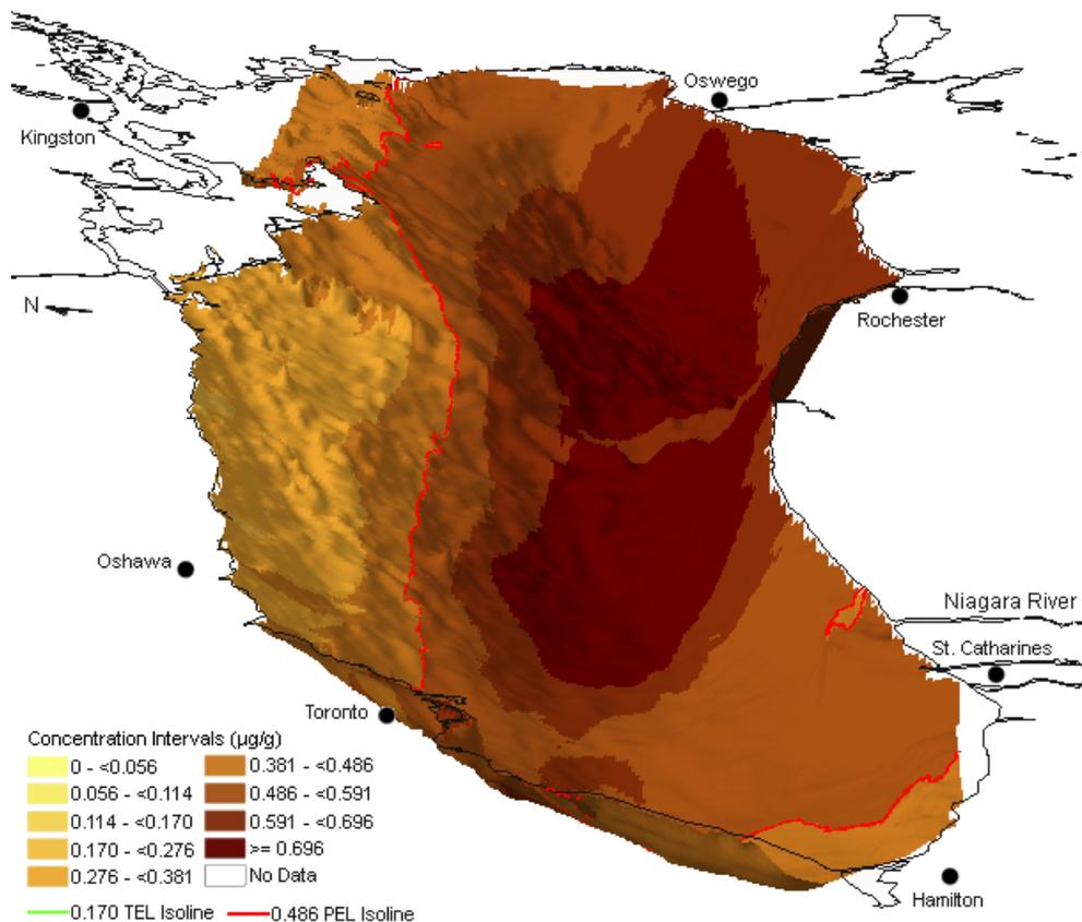
**Fig. 10:** Lake Ontario Kriged 1998 Mercury Contamination with Bathymetry
