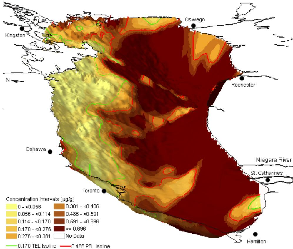
**Fig. 9:** Lake Ontario Kriged 1968 Mercury Contamination with Bathymetry
