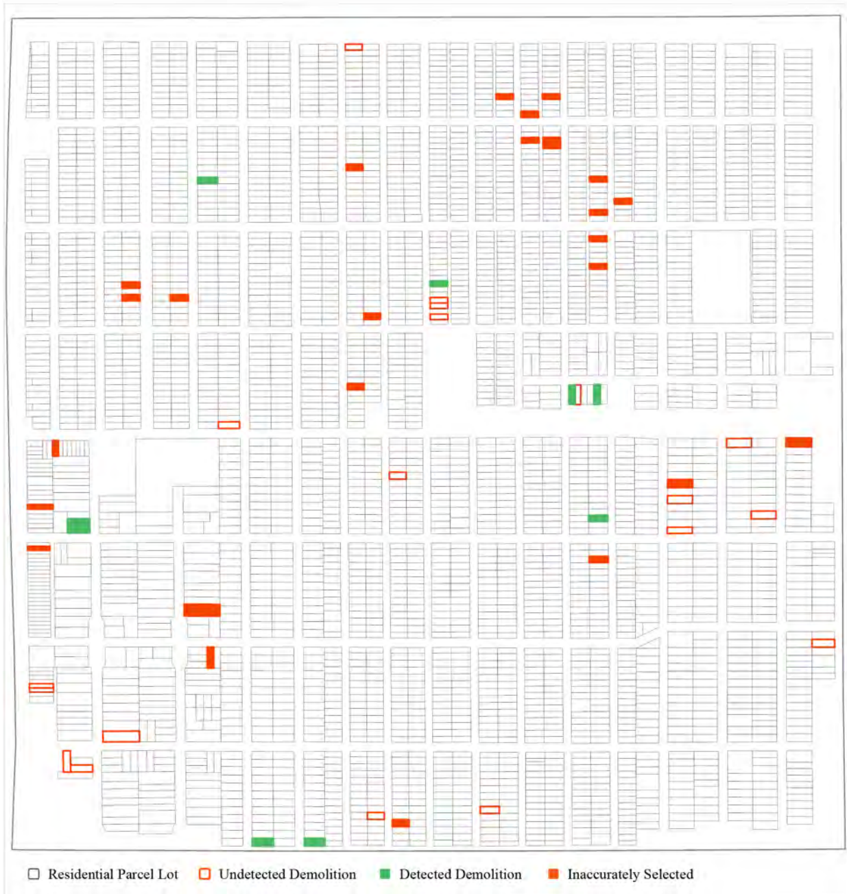
Figure 5.13: Crary/St. Mary (low residential demolition rate) – correct/incorrect change detection (based on 25 square metre structure threshold)
