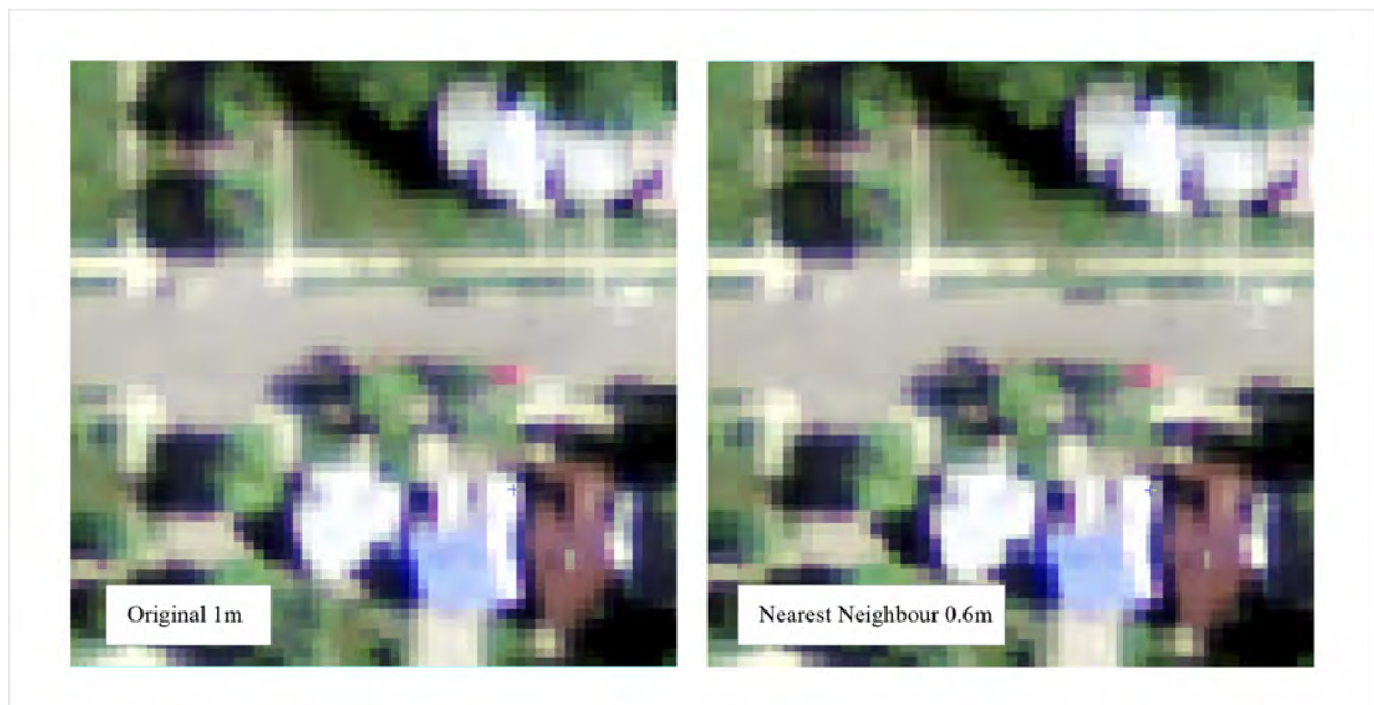
Figure 3.2: NAIP 2014 resampling from 1m to 0.6 m with Nearest Neighbour method
