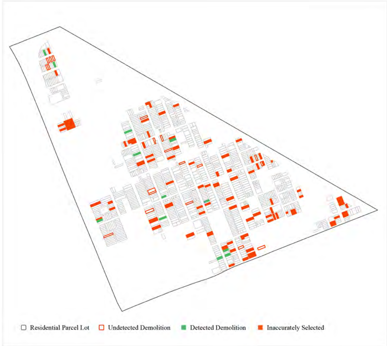
Figure 5.14: Core City (median residential demolition rate) – correct/incorrect change detection (based on 25 square metre structure threshold)
