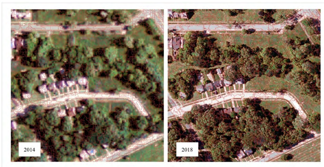
Figure 5.1: Tile extent - image segmentation outcomes in 2014 and 2018 based on Blue and NDVI channels, scale of 5, shape of 0.1, and compactness of 0.9
