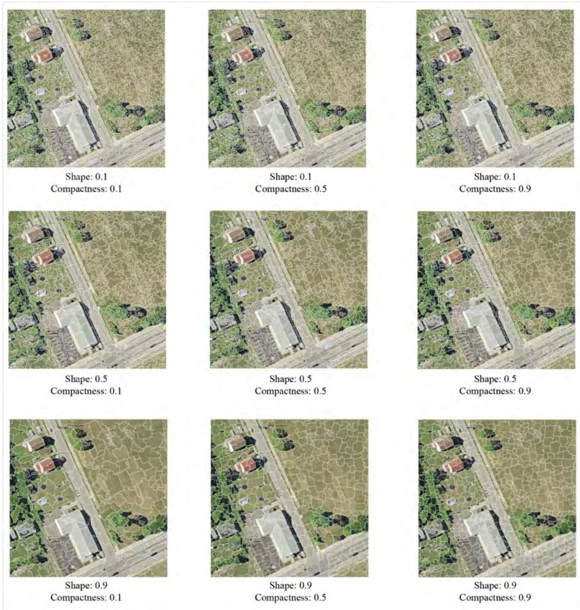
Figure 4.4: Image segmentation shape and compactness matrix example. Based on the RGB bands, with a scale of 5.
