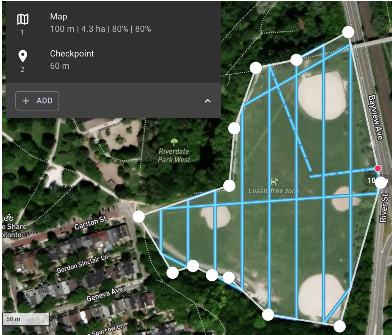
Figure 3-7 Riverdale Park West Flight Plan with mission details. (100m with 80% image overlap)
