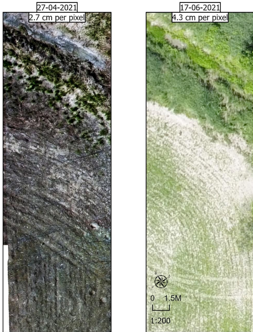
Figure 6: Zoomed-in images of the flights performed on April 27th and June 17th to compare the change of resolution caused by the increased altitude.
