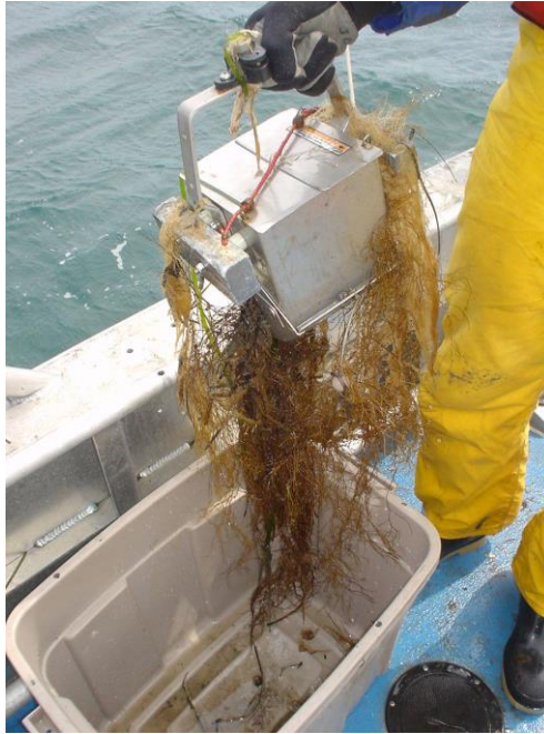
Figure 5: Sediment sampling using an Ekman Grab. Occasionally samples could not be obtained due to interference of seaweed and hard bottom types.
