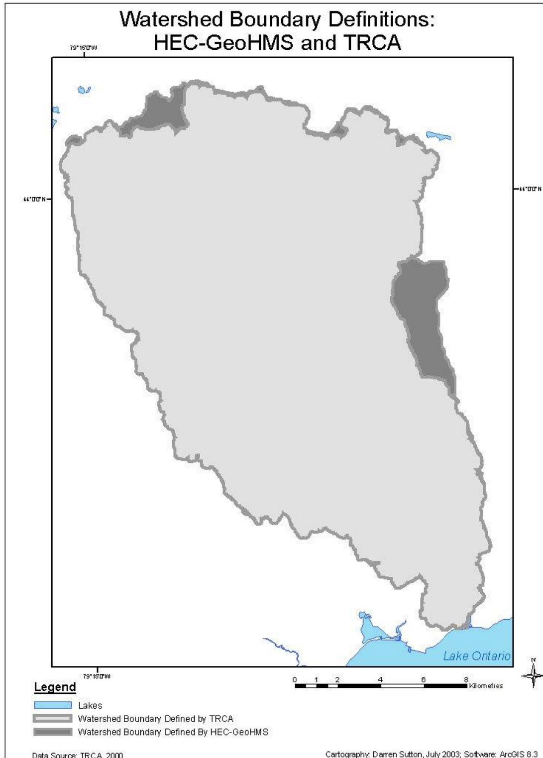
Figure 3.3: Difference Between Duffins Creek Watershed Boundaries Defined by the TRCA and HEC-GeoHMS
